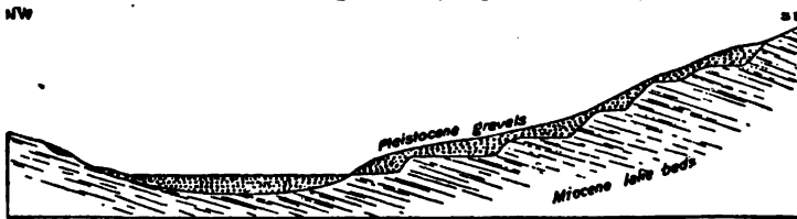
Fig. 57. Bench and valley placers. Section across Rye valley, Blue Mountains, Oregon. After W. Lindgren.
